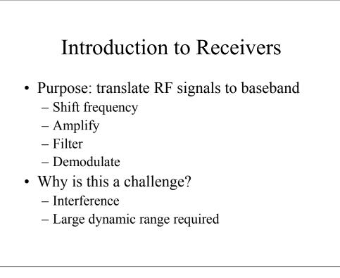
Many receivers must be capable of handling a very wide range of signal powers at the input while still producing the correct output. This must be done in the presence of noise and interference which occasionally can be much stronger than the desired signal.
